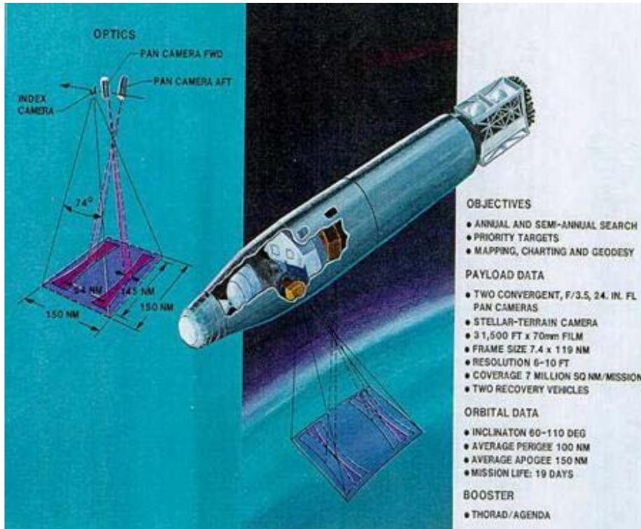
Fig. 17web-9. Description of the Corona Payload, the First Known Space-based Observational Payload for Intelligence Collection.
